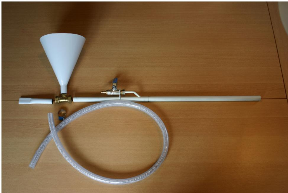
The simplest way to dose MARISOL SR into boiler fire-side:
